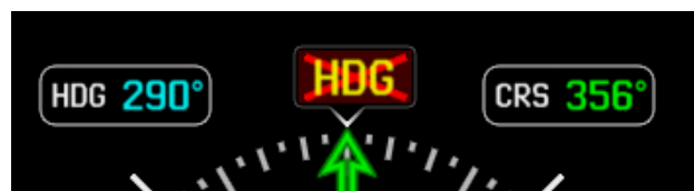
Figure 5-4 – Heading Failure Indication
