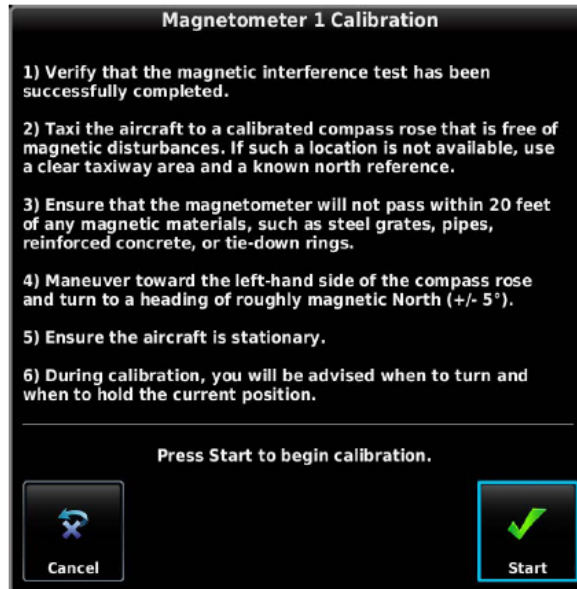
Figure 7-5 – Magnetometer Calibration On-Screen Instructions
